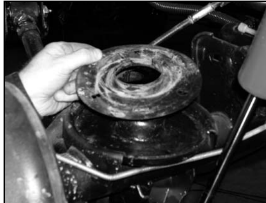
Figure 13.3: Removal of Lower Mount Insert
