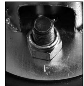
FIGURE 11.5 FRONT UPPER MOUNT MARKED WITH “F” POSITION THIS TOWARDS THE FRONT OF VEHICLE
