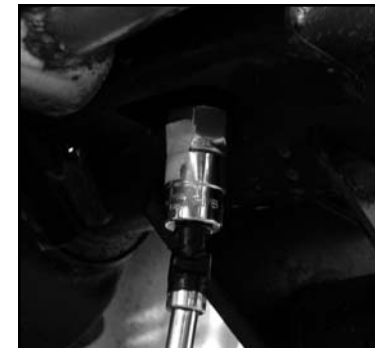
FIGURE 12.5 ADDITIONAL METHOD OF STARTING NUT ON FRONT LOWER RIGHT MOUNT
