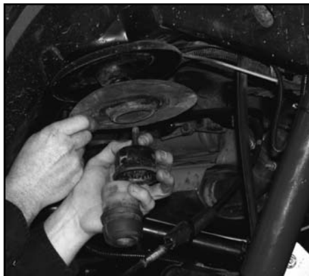
Figure 13.2 Removal of upper hardware
