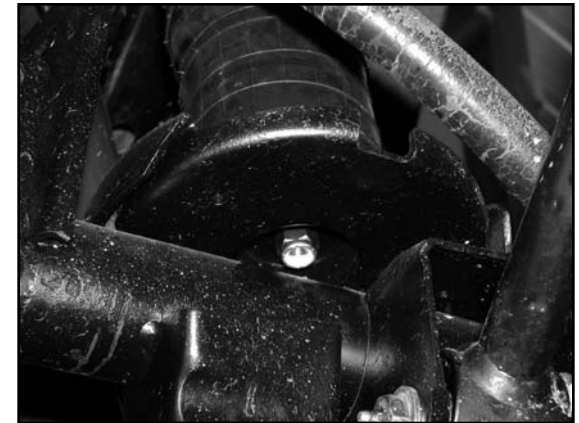
Figure 14.4 Install nut on lower stud
