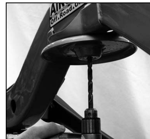
Figure 13.4 Drill upper bumpstop mount threads to 3/8"
