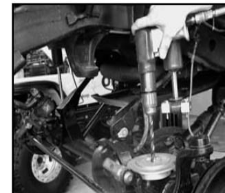
FIGURE 10.3 PLACE AiROCK LOWER FRONT MOUNT OVER SPRING PAD AND MARK FOR DRILLING 1/2" HOLE
