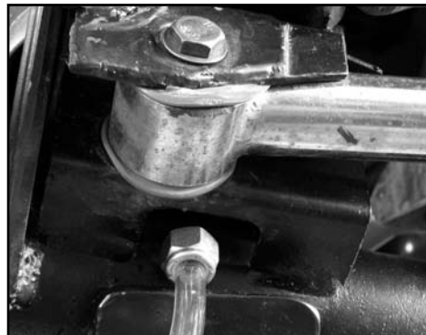
FIGURE 12.4 UTILIZE NUT INSERTION TOOL TO START NUT ON STUD
