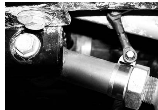
FIGURE 8.3 ROUND CONTROL ARM SHOWN WITH SENSOR LINKAGE MOUNT INSTALLED. NOTE THE LINKAGE BRACKET IS AT THE JAM NUT EDGE.
