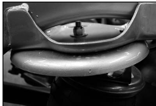
Figure 14.3 Install washer and nut on top mount
